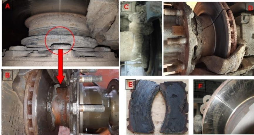
Figure 2. The main defects identified in the braking systems: A- cracks in the brake disc in the area of the fixing screws; B- breaking the disc due to cracks; C- deposits that block the movement of caliper; D, F- thermal overload on disc surface; E- overloads effects on the brake pads.
